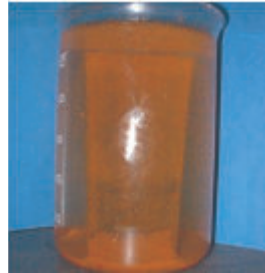
After 1500 hours Mild steel immersed in sea water without Vapro 844L.
