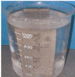
After 1500 hours Mild steel immersed in sea water with 700ppm of Vapro 844L.
